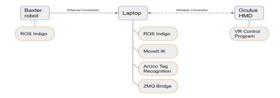
Figure 2: A high level overview of the system, with both hardware (square blue outline) and software (capsule orange outline) components shown.
