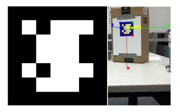
Figure 3: An example of ArUco tag number 503 (left) being identified via a usb webcam (right).
