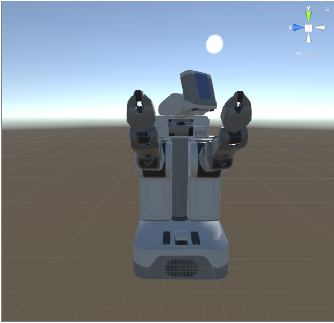
Fig. 3. An image of the PR2 robot visualized in Unity from the URDF Parser of ROS Reality.
