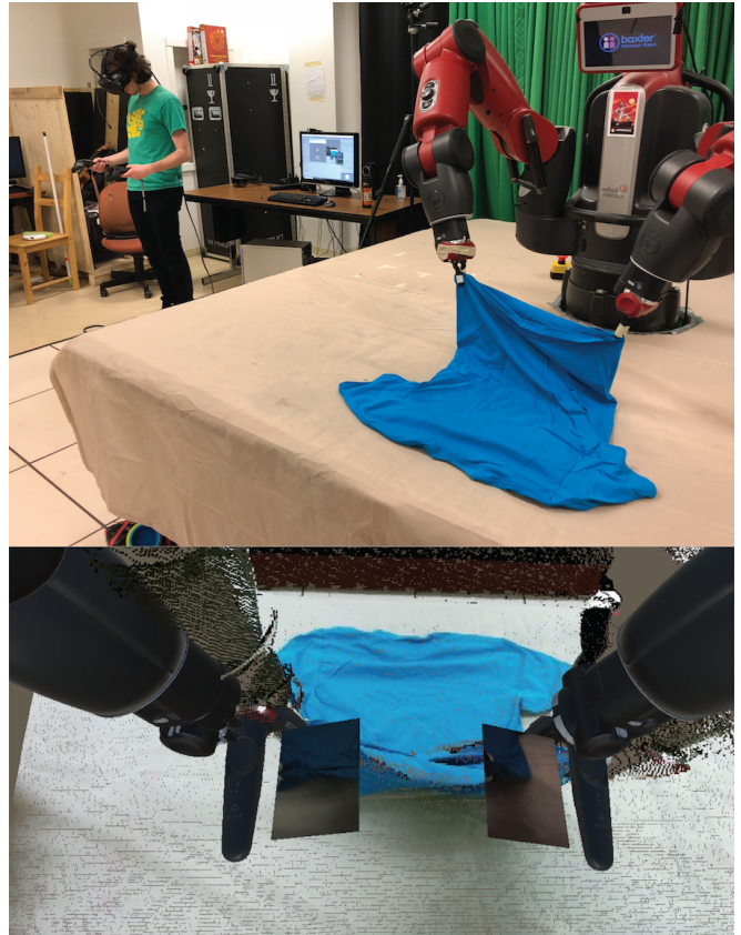
Fig. 1. Top image: An operator using ROS Reality VR to teleoperate a Baxter to fold a shirt. Bottom image: View of scene from VR headset. Note a point cloud, mesh model of robot, VR controllers, and wrist camera feeds from robot are all visible to the user.
