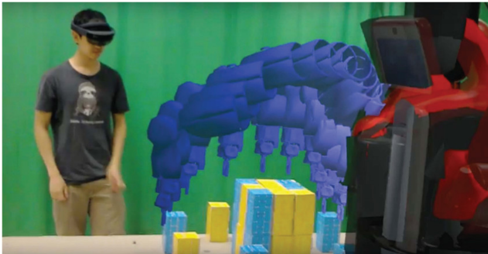
Fig. 1. An image captured directly from the MR Headset of a user viewing a robot trajectory.
